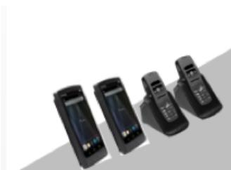
Spectralink phones can be a **shared resource**, utilized as, and when needed, across shifts with individual logins. The batteries and hardware are built to last, with over **10 hours talk time** from one charge, and spare batteries can be charged at the same time.
